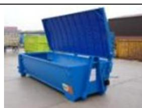
Skips with a hydraulic roof have a fail-safe pin for use when the roof is open to prevent it closing accidentally. This pin is removed before the close valve is operated. The roof has a locking device to ensure it remains closed when the skip is in transit.
