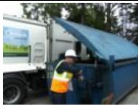
At some Surrey Waste Management sites, a member of the collection crew is required to open the hydraulic lid of the skip in order for the driver to deliver the food waste load. A site requirement is the wearing of a hard hat while on site and the crew member opening the lid must comply with this.
