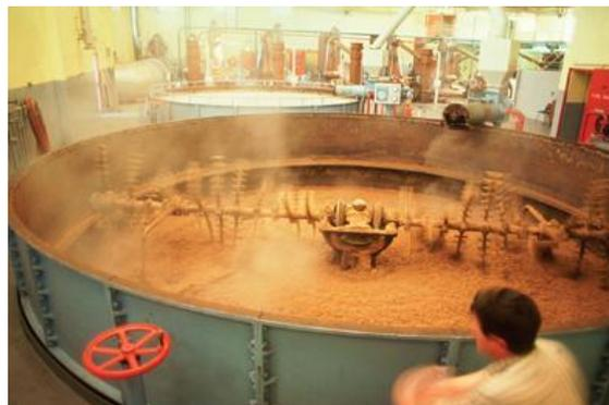
Image 2: **Mash tun.** Malted barley or grain is mixed with hot water in a mash tun
