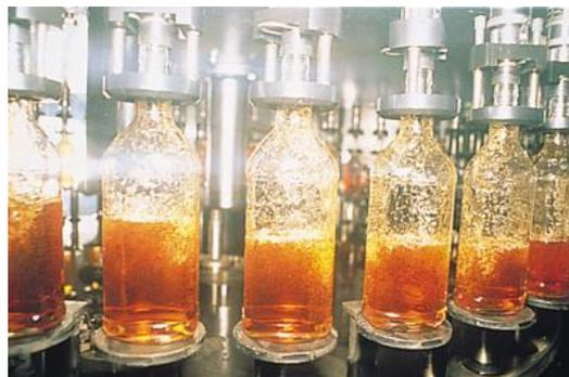
Image 1: **Bottling line.** Whisky is a premium product and is frequently packaged in heavy glass bottles
