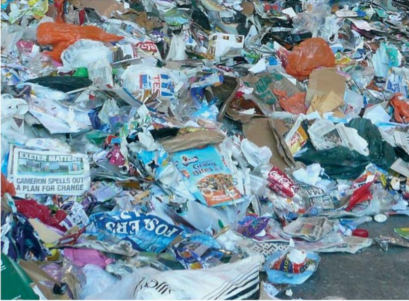
Input stream of co-mingled recyclates prior to sorting by the Exeter MRF
