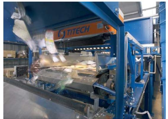
The TiTech uses high-precision jets of pressurised air to blow contaminants off the line
