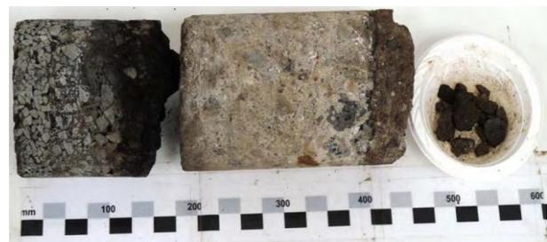
**A66 pavement core (tar bound binder course can be observed between 100mm - 200mm). Photo courtesy of PTS Ltd**
