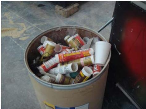
Sealant cartridges segregated within the factory for shredding and recycling
