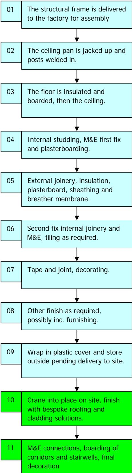
Caledonian modules are made from fully welded steel frames. Depending on the module type, the steel frame chassis may be laid out for a longitudinal plan (in which bedroom modules are placed either side of a corridor module) or a transverse plan (in which modules incorporate a bedroom either side of a short section of corridor). Finished module height rather than length and breadth is the principal transport restriction.
