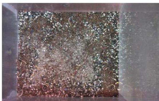
Fig. 8: Top view of jig compartment showing the bottom layer after the upper layers have been removed
