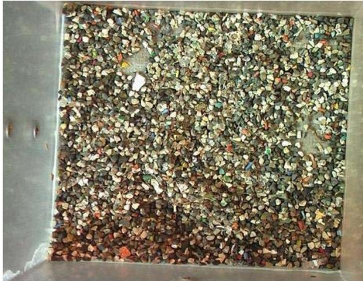
Fig. 13: Top view of jig compartment showing the bottom layer after the upper layers have been removed
