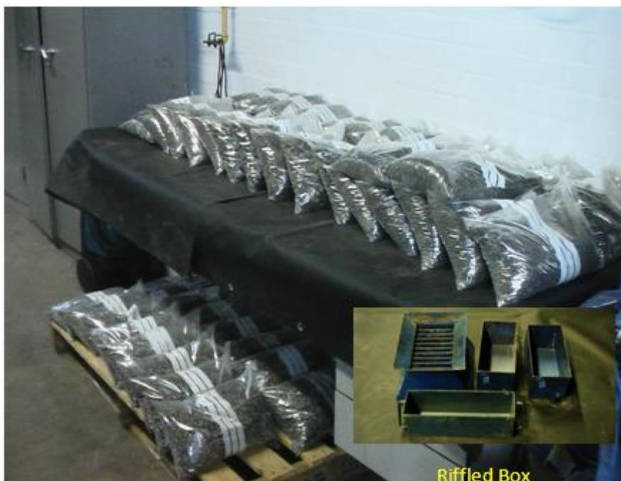
Fig. 3: Riffled Samples
