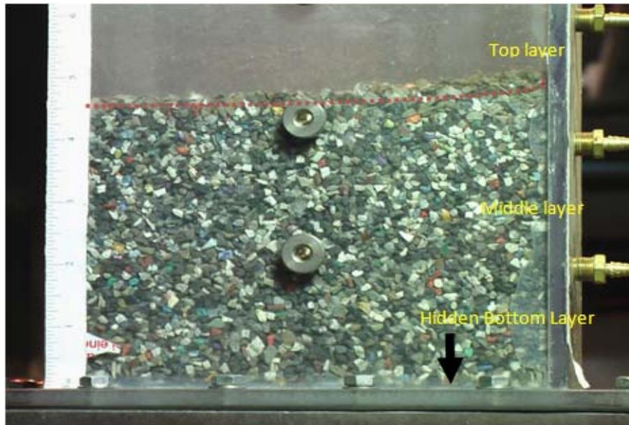
Fig. 9: Side view of jig showing the three layers after separation
