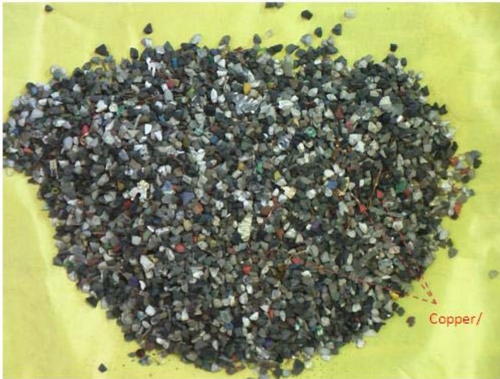
Fig. 12: Bottom layer (small amount of copper/metal)
