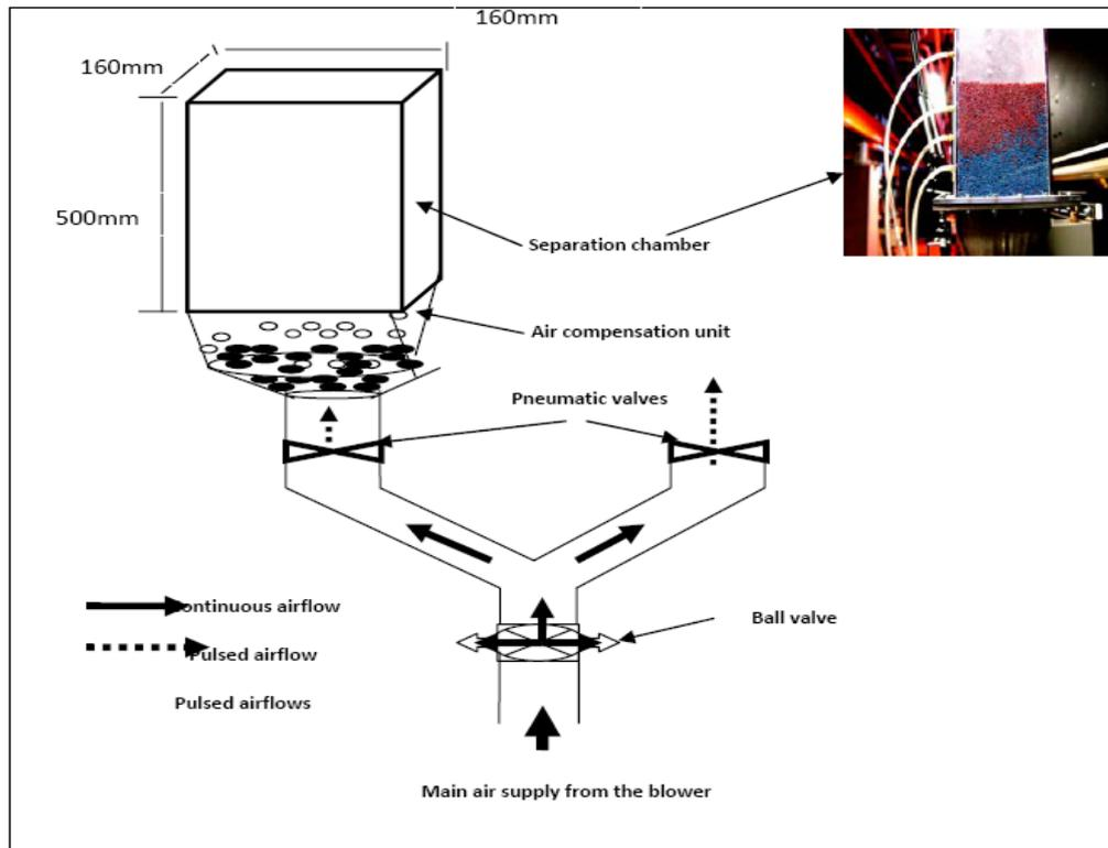
Fig. 2: Schematic of the pneumatic dry jig and separation chamber
