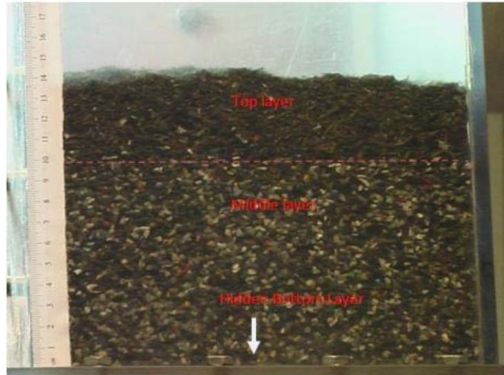
Fig. 4: Side view of jig showing the three layers after separation
