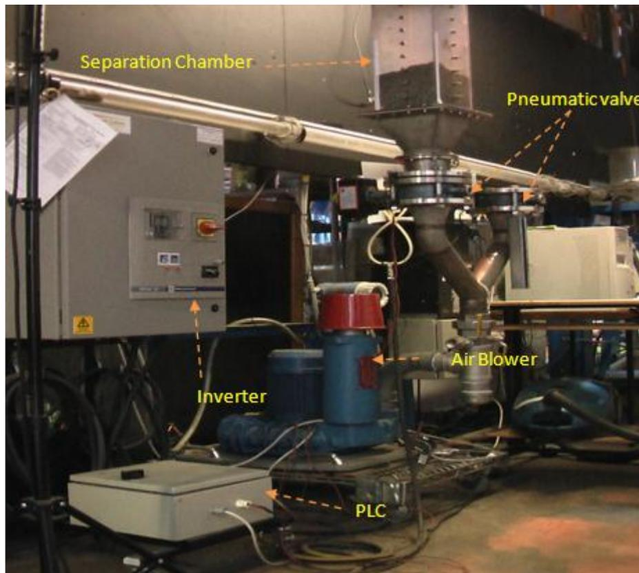
Fig. 1: Batch scale experimental pneumatic jig
