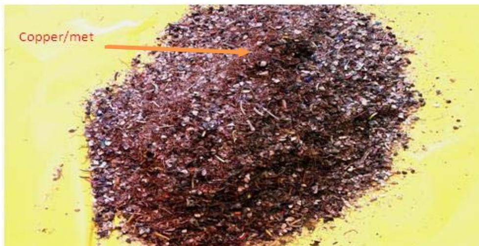
Fig. 7: Sample 1 – bottom layer (copper/metal rich fraction)
