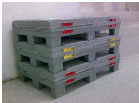
Plastic folding box pallets owned by Whitecroft Lighting at the London Construction Consolidation Centre (top) and collapsed empty pallets stacked for return to supplier (below) (From WRAP, Case Study: Material Logistics Planning, Barts Hospital. London, March 2010)
