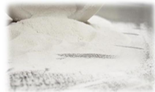
The powder is heated with water and natural additives. The water is used as a plasticizer. This produces a dull-white, dough-like mass. The production process, which has been operational since 2014, is akin to a large noodle making machine.
