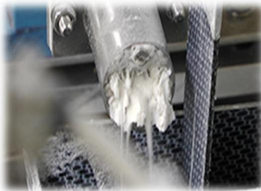
The casein mix is pressed in a continuous extrusion process through a specially shaped spinneret.
