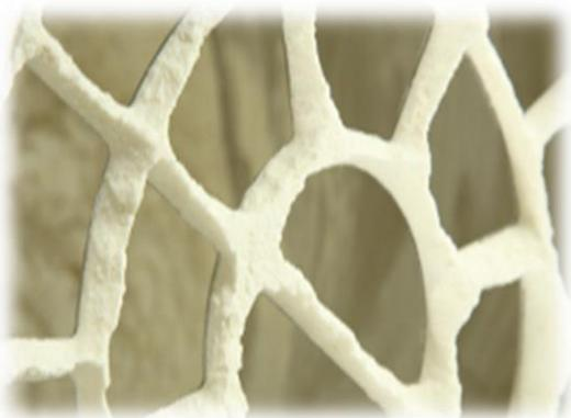
Since the process temperature is 80°C, the special properties of the milk can be maintained. The extruded filaments are dried naturally before being cut into individual fibres.
