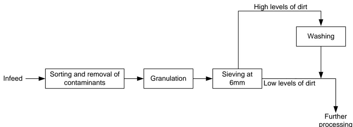
The three feedstock materials were granulated and sieved through a 6mm mesh screen in preparation for producing panels, as can be seen in **Figure 5**. The pulverised polyethylene skin material was passed through a 500 micron mesh screen in order to ensure a smooth surface for the panels.
