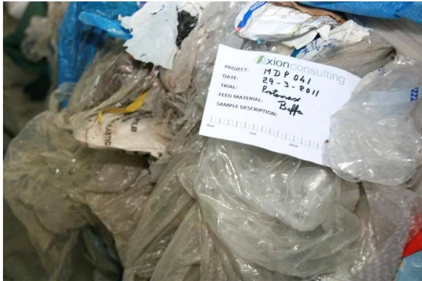
**Figure 2** Sainsbury's film feedstock material
