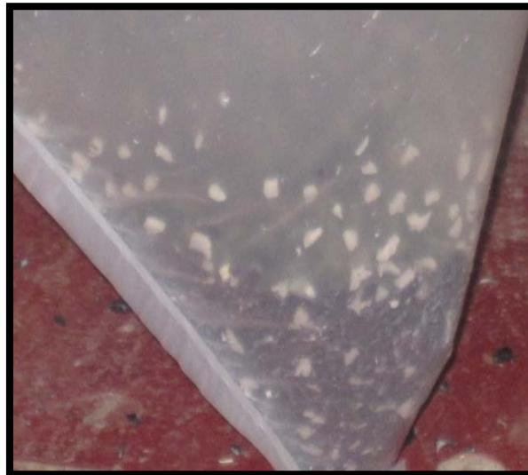
Figure 11: Apparent elastomer-PS separation
