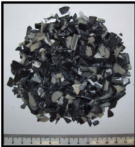
Figure 8: Granulated PP Sprues
