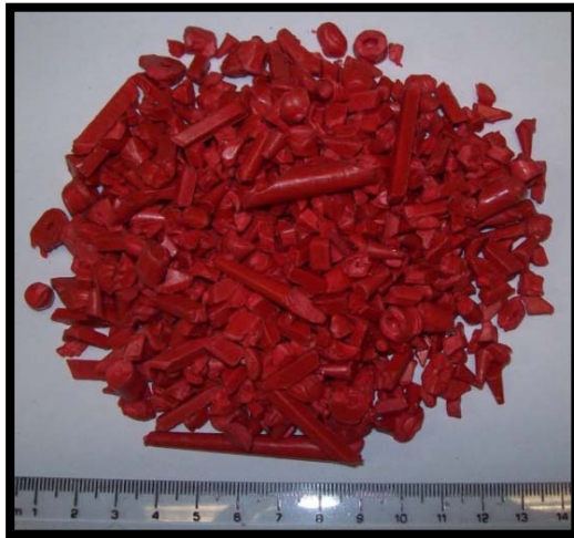
Figure 8: Granulated PP Sprues
