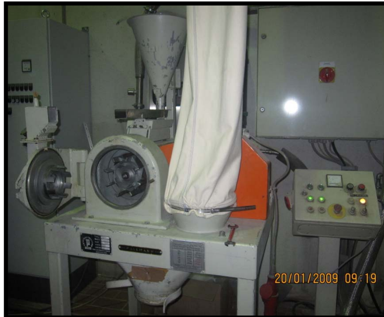
Figure 2: Photograph of the PALLMANN - PXL18 Mill
