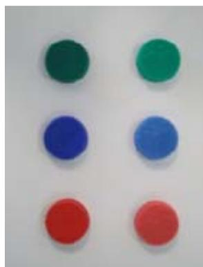
Optical sorting trials conducted at Greenstar-WES and Closed Loop Recycling have confirmed that tinted caps can be identified and sorted with existing optical sorting equipment. Tests at Robert Wiseman Dairies have confirmed that tinted caps can be recognised by colour recognition systems with the dairies. It is recommended that further trials are done at specific dairies prior to implementing this to ensure that the particular equipment in operation can identify tinted caps.
