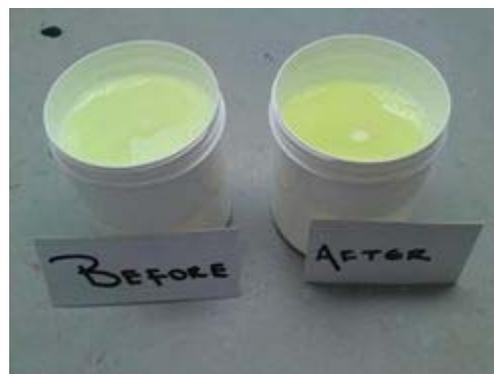
A follow up test was then made using printed Polypropylene labels from Systems Labelling, made using similar UV-curing inks. The aim was to assess the possible residual colours after bleaching of typical commercial labels, however it should be noted that the prints were un-laminated versions of labels which would normally be laminated.
