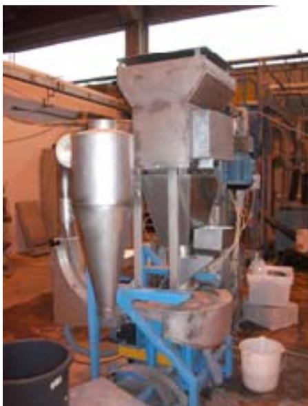
At the UK reprocessors colour sorting removes colour contamination from the HDPE flake prior to the extrusion step. However, during this trial, a colour sorter was not available, so an additional air separator was used to help remove label/cap fragments.
