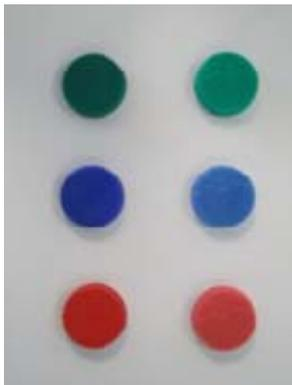
Tests at reprocessors and in a dairy have confirmed that the tinted caps can be recognised by colour recognition/sorting equipment as effectively as the current coloured caps.
