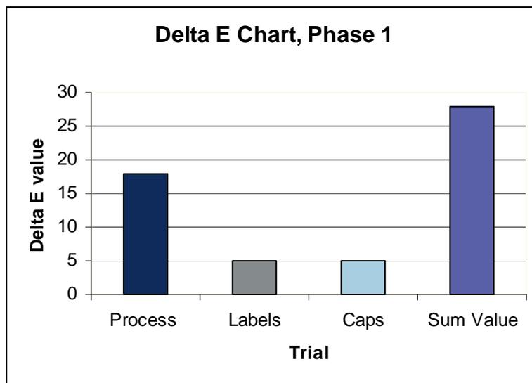
Note: The level of coloured cap material getting into the extrusion process is critical. The level of cap contamination in this analysis was 0.2% of the material extruded being cap material.
