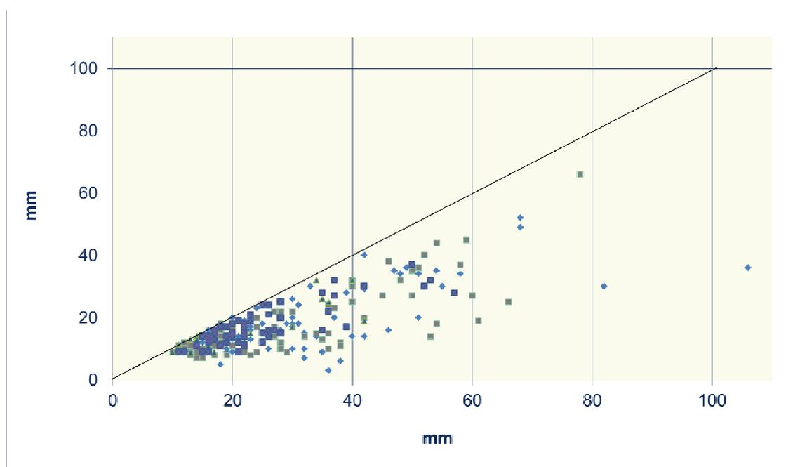
Figure 9 shows that there is a spread of different shapes (based on the ratio of height to width) of particles. There is a cluster of square and spherical particles i.e. those with height and width of similar dimensions,
