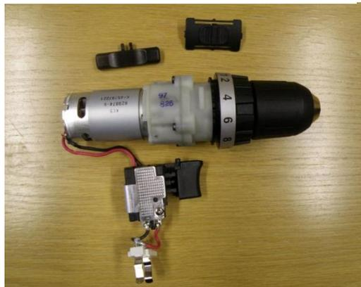
**Figure 10** Soldered joints that restrict component replacement
