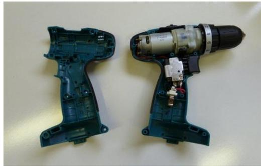
**Figure 9** Switch assembly, motor, gearbox and chuck
