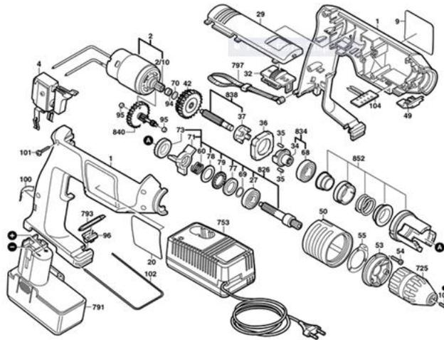
The key parts to consider for price and availability are batteries, switches, motors, chucks and gear boxes. To give some examples for one of the professional drills (costing around £130), a switch would be less than £3, a keyless chuck around £20, a DC motor between £10-25, a gear assembly £20-40, and a Ni-Cd or Ni-MH 14.4v battery - over £50.
