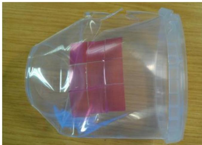
The crushing meant that when placed on the belt the diffraction pattern was formed away from the screen due to the angle of the packaging. It was therefore not captured by the camera and was not able to be detected. This would have to be taken into account during the design of a commercial sorting unit and could probably be addressed by covering a larger area with the screen.
