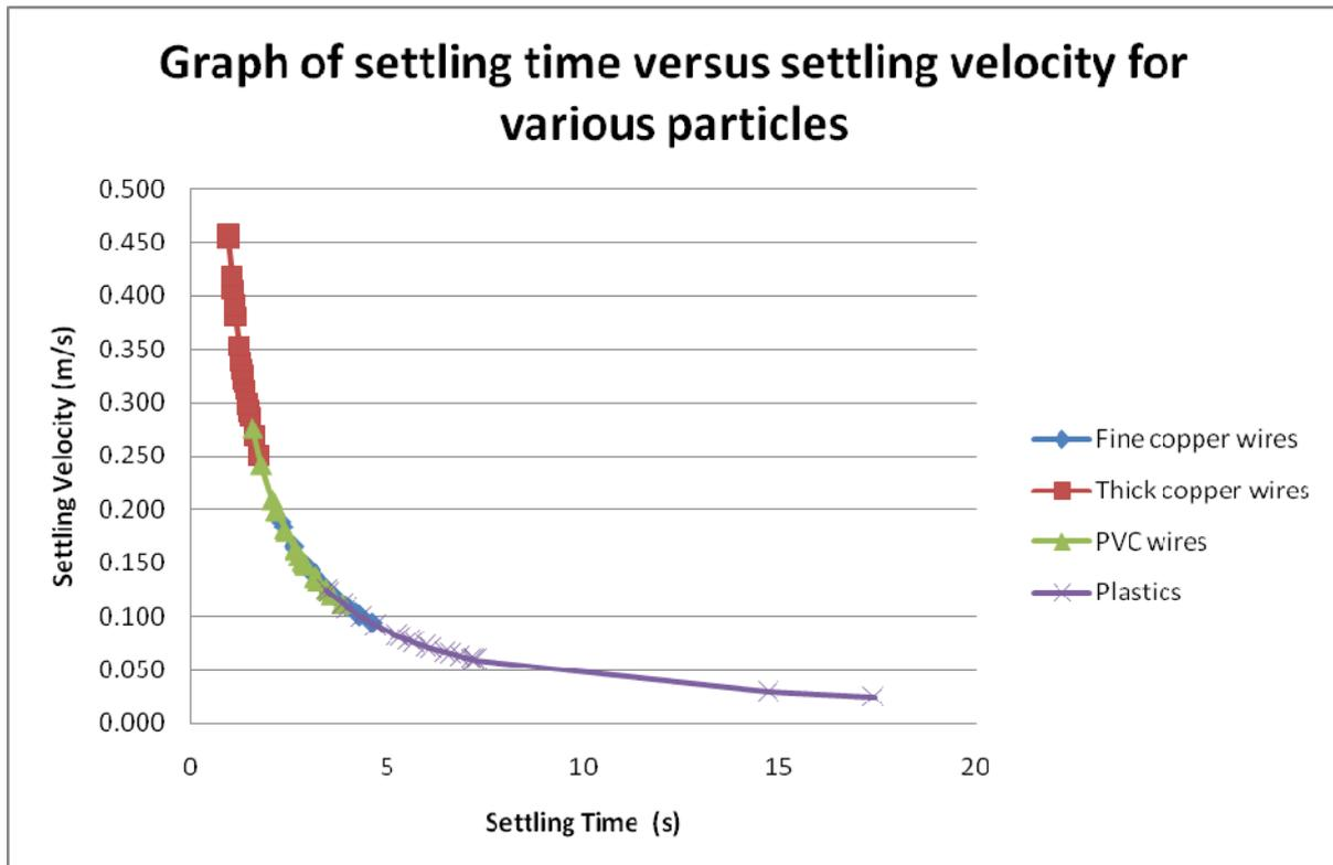
The information on the settling velocities will prove useful when adjusting the settings of the kinetic gravity separator to obtain the most effective separation.
