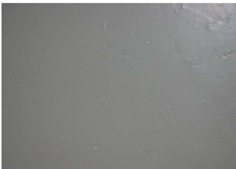
Figure 9 Surface irregularities due to trapped contaminant particles
