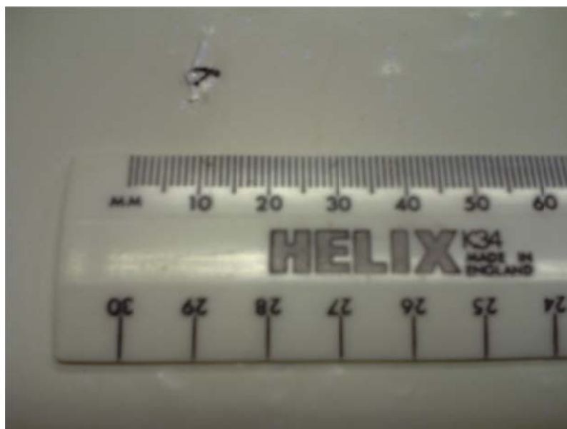
Figure 7 Puncture in white plastic film surface coating caused by hot contaminant particle in extruded material
