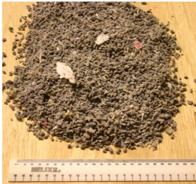
Figure 3 Agglomerated film material (minimal pick)
