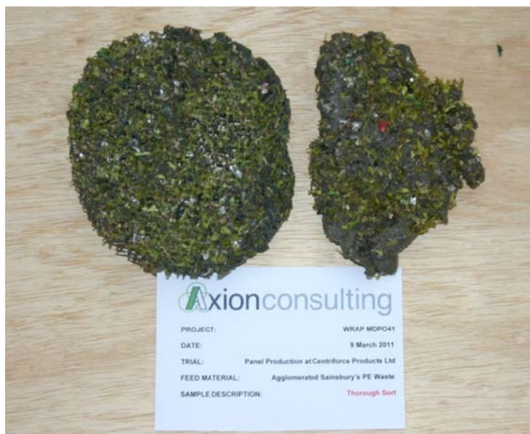
Figure 8 Fouled screen removed during extrusion of thorough pick feed material
