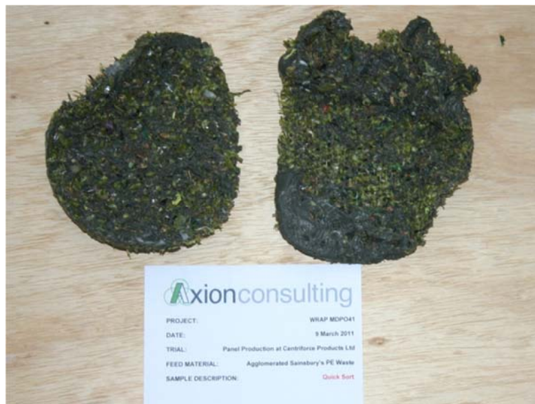
Figure 9 Fouled screens removed during extrusion of minimal pick feed material
