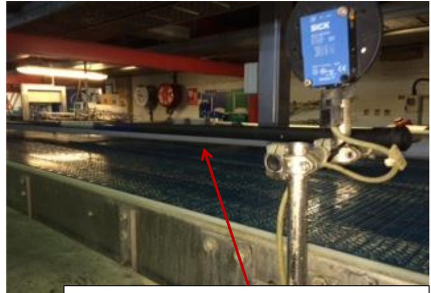
The "fishing rod" guide installed on the line – the guide is supported at one end only allowing the rod to flex against product in transit and prevent falls
