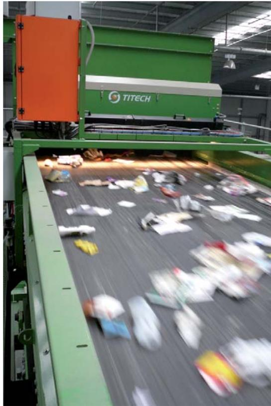
Mixed plastic approaches a near-infrared optical separator
