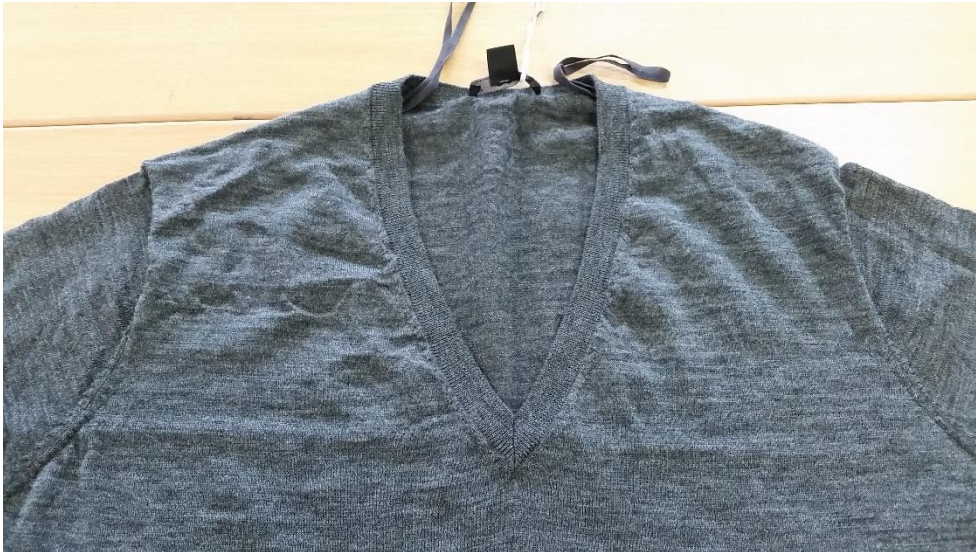
Original grey after one wash. Detail around neckline shows slight cockling.
