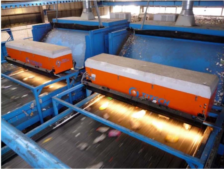
Figure 2 NIR sorting equipment similar to that at the Biffa MRF Trafford Park
