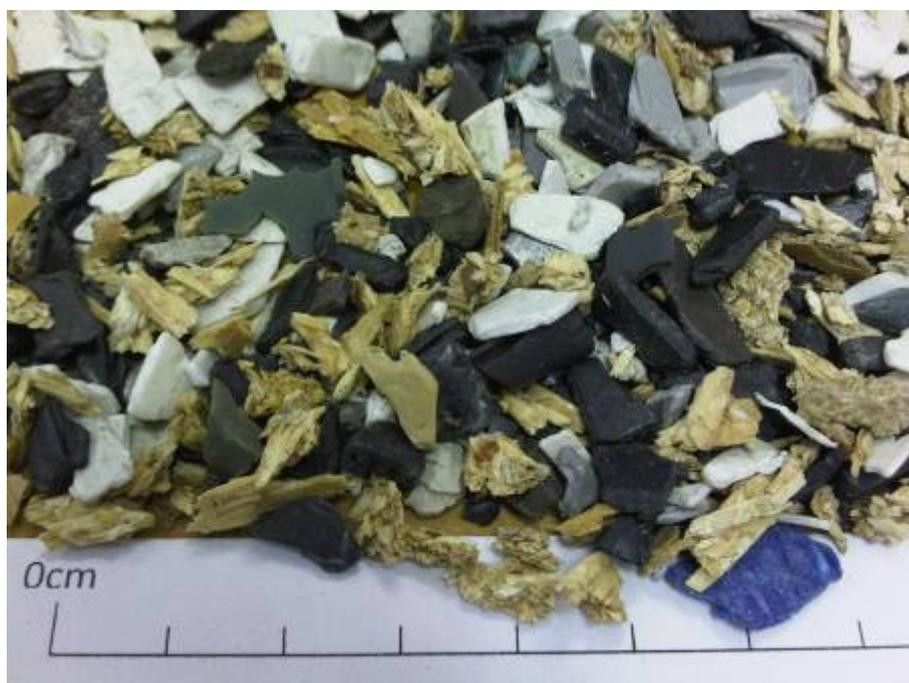
*Figure 30: Photograph of trial 5 light fraction*
