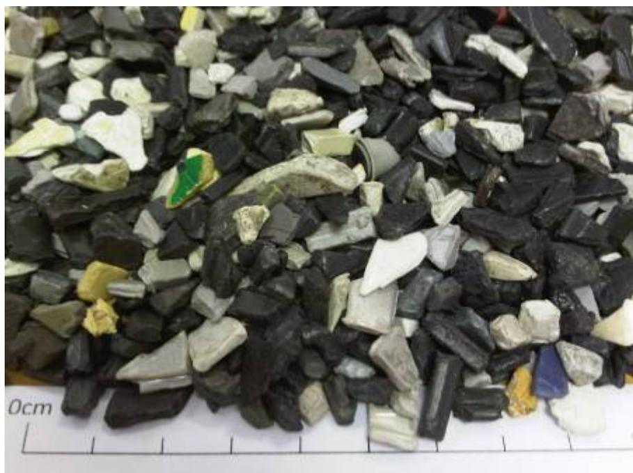
*Figure 16: Photograph of trial 2 heavy fraction*
