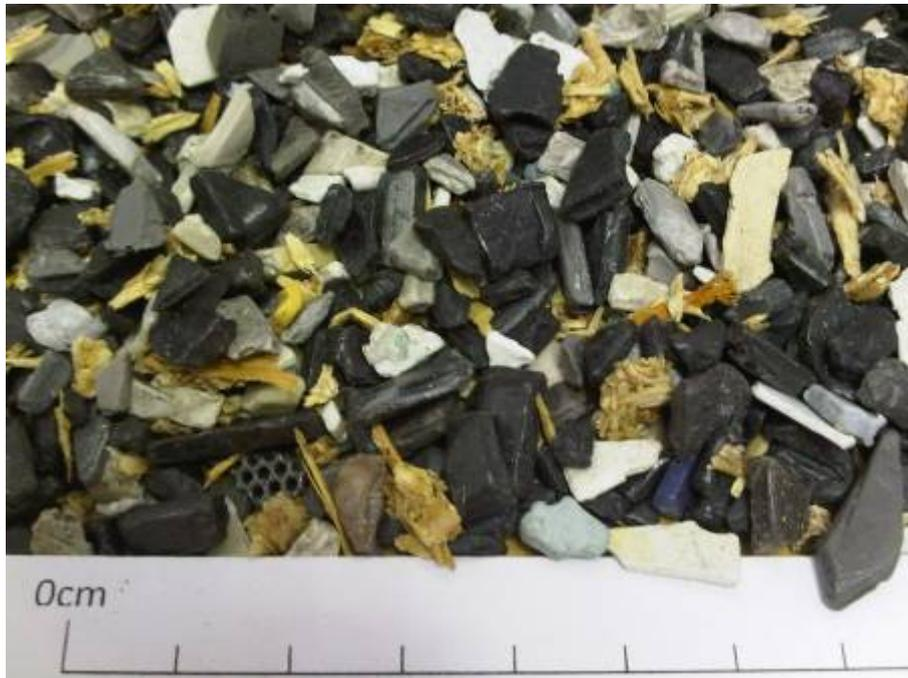
Figure 13: Photograph of trial 2 feed material, 3-8mm fraction
