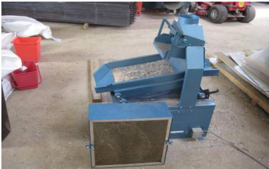
*Figure 4: Destoner showing Light Output on left and Heavy Output on right*
