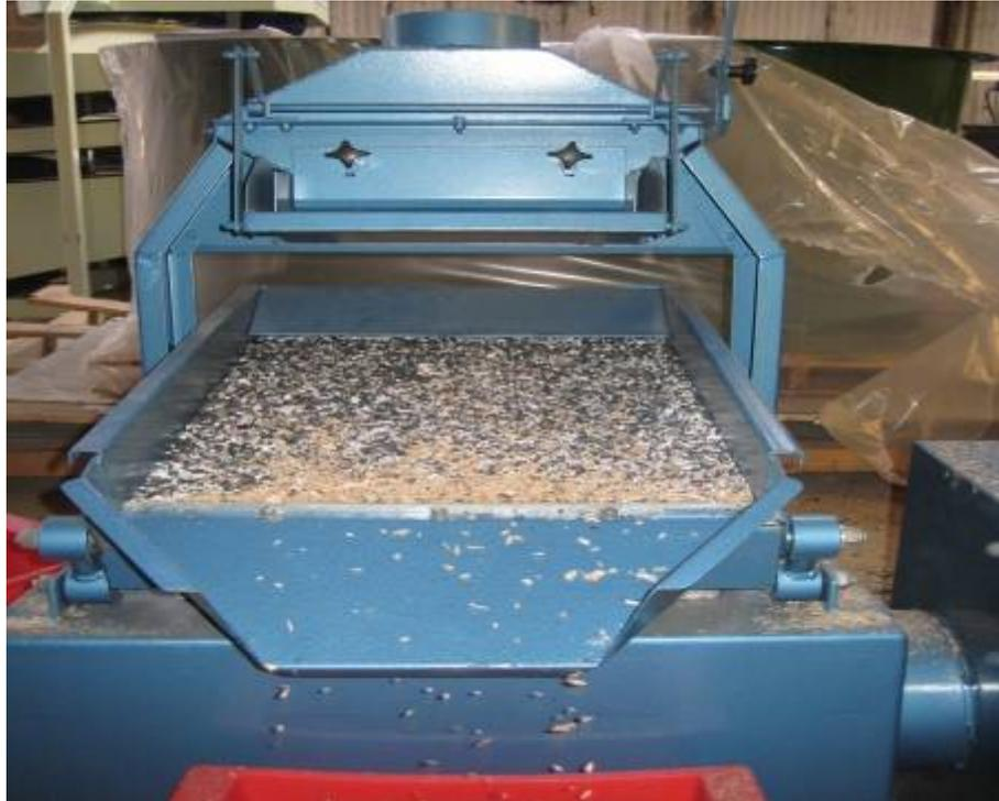
*Figure 5: Light Output End of Destoner*
