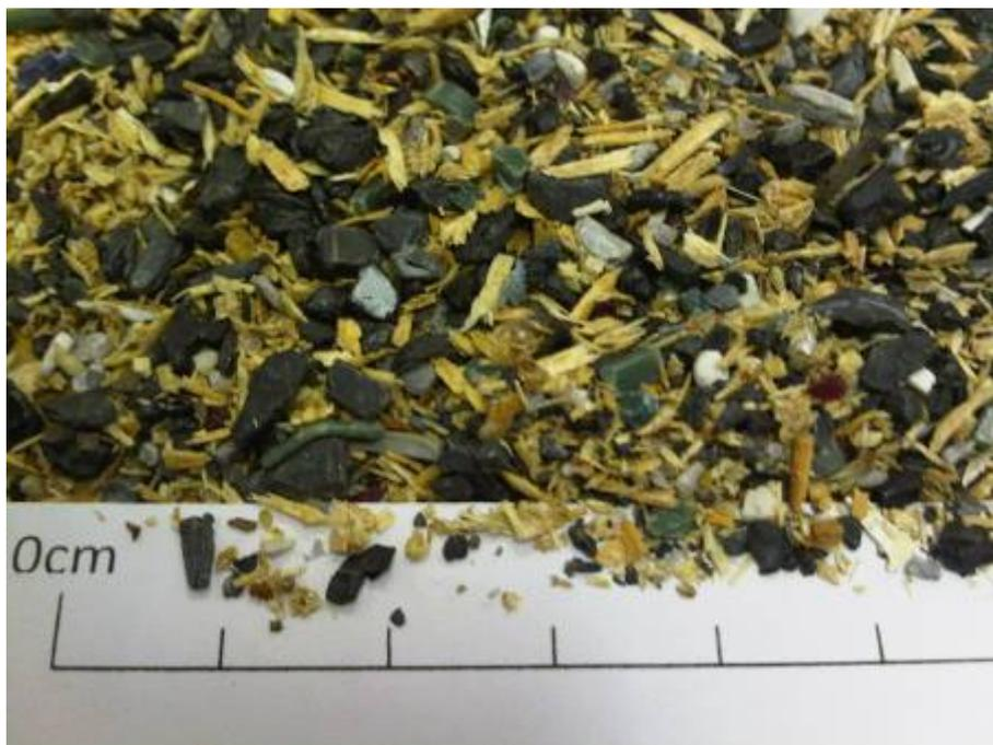
Figure 6: Photograph of trial 1 feed material, 0-3mm
