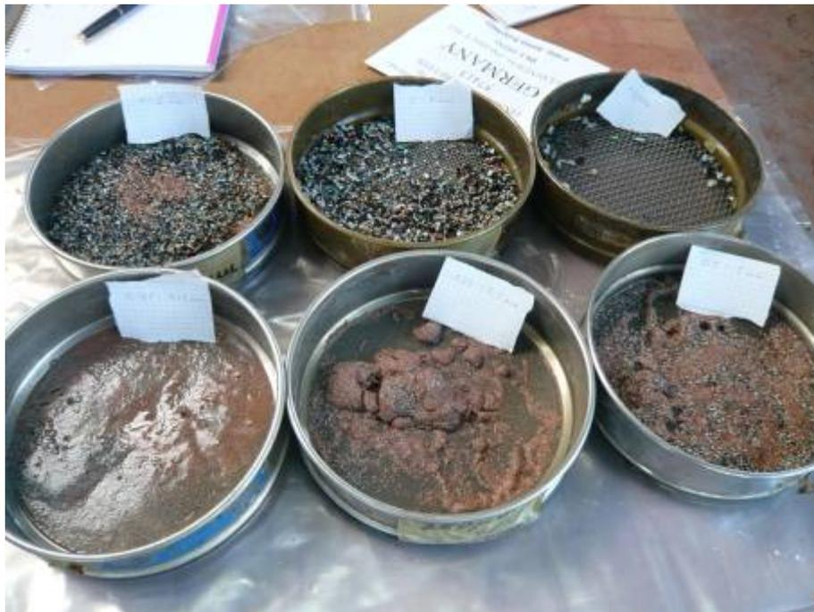
Figure 7: Trial 2 heavy fraction sieved into 6 fractions
