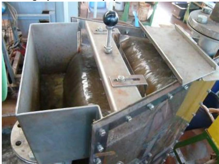
*Figure 2: Top view of the Miniflux separator showing the two separating sections*
