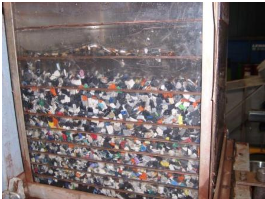
Figure 14: Photograph of the wet jig in operation with the mixed plastic material
