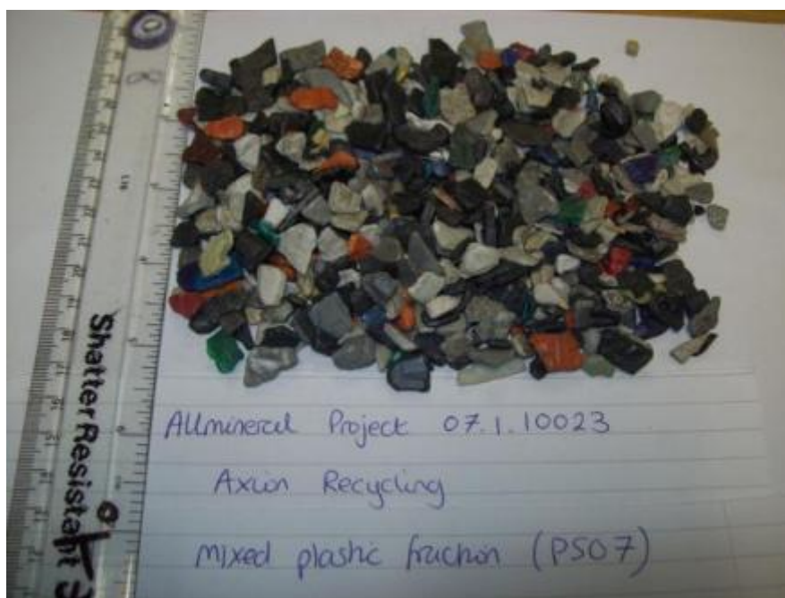
Figure 13: Photograph of mixed plastic feed material
