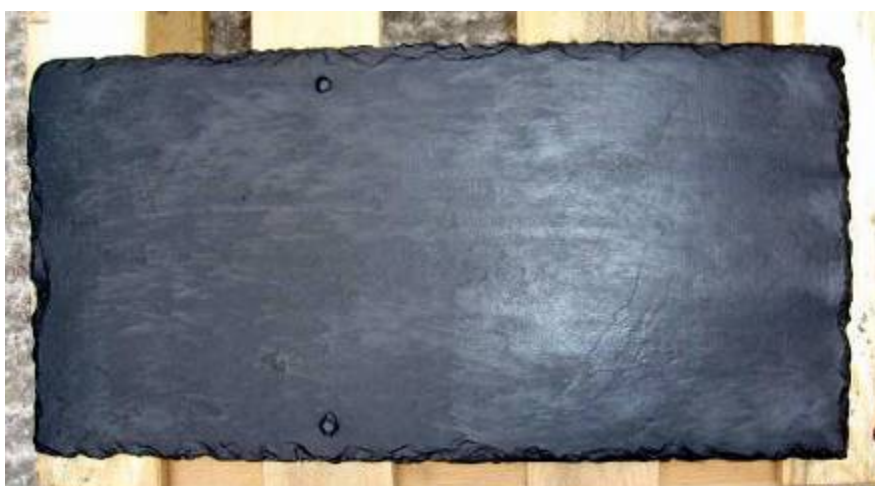
Fig. 5: Injection moulded 40wt% rubber-PP composite replica roofing slate
