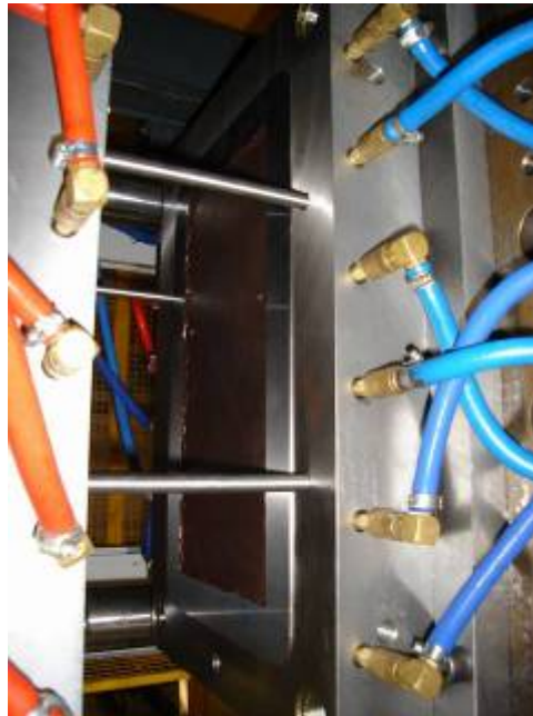
Fig. 2: Injection mould tool in-situ, open
